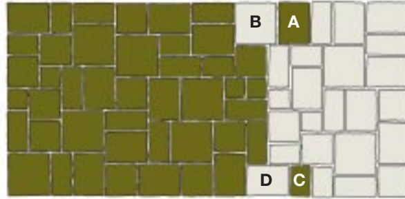
Large patio pack (10.2m 2 ) and small patio pack (5.5m 2 ) with random laying pattern
