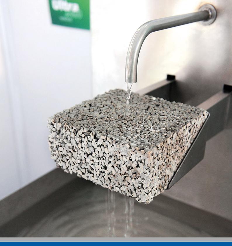
Hydromedia Fast draining engineered concrete
