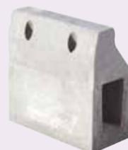
Blending practicality with aesthetic appeal, Mini Highway is a two-part integrated kerb profile and linear drainage system offering efficient drainage capability. Comprising a base unit and kerb profile top unit with two elliptical holes, the kerb incorporates multiple inlet holes along its length for fast water take off.
