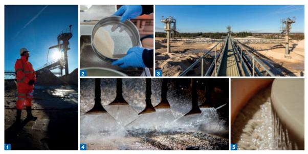
Each tonne of sand is washed with circa 3000 litres of water fully recycled through our water recovery system. The whole system recycles circa 800 million litres of water per annum.
